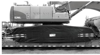
Cloth covers designed to wrap the excavator tracks on the floats while travelling. The different sizes are distinguished by a different color code (blue = small, red = medium, black = large). The cover surrounds and encloses the excavator tracks to counter the possibility of the loss of residue while being transported. The installation of the cover is done in a short time. An aluminum storage box is optional.
